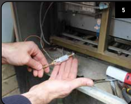
5 Release pressure on the thermocouple testing device spring only.
