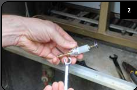
2 Fit the end of the thermocouple into the tester. (If you need to, use the universal bush provided, you may need to gently flatten a section of the thermocouple tube to slip the bush on)
