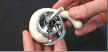
1. Roll out and place around plug and washer
