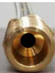
Reduced internal bore, restricting gas flow
