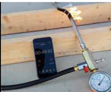
Rubber core is easily ignited
