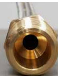
Reduced internal bore, restricting gas flow
