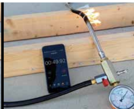
Rubber core is easily ignited
